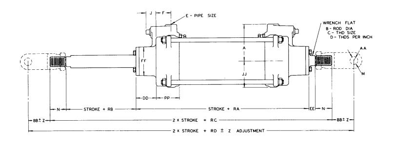
This cylinder can use foot mounts, flange mounts, or trunnion mounting.
